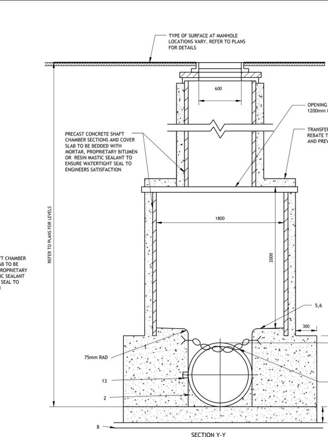
**MANHOLES 3m TO 6m DEEP (DETAIL USED ON ULVSS CONTRACT)**
