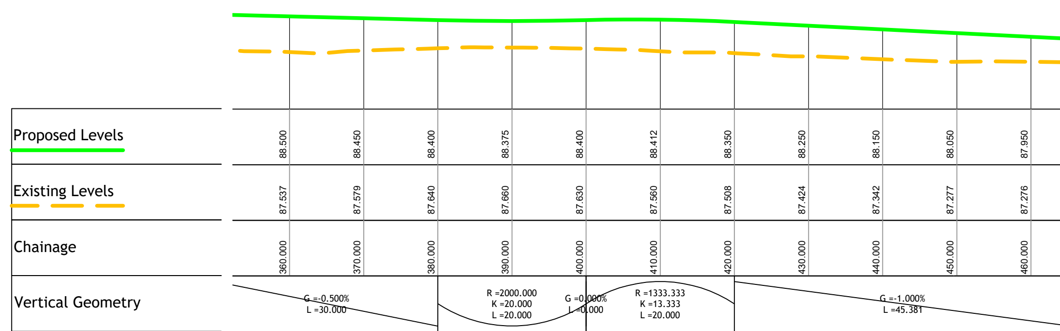
STREET - 2A - (CONTINUED) - LONGSECTION SCALE: H1:500, V1:100 DATUM: 85.00
